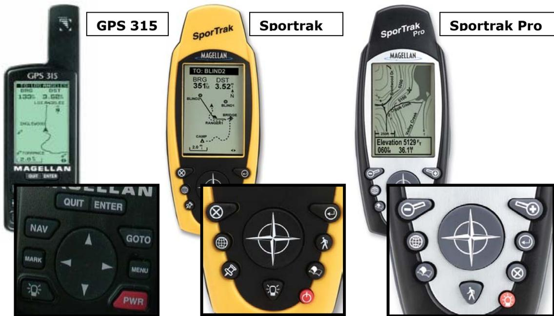
As the GPS unit improves its features and interface, some of its buttons has slightly been repositioned and redesigned. For the purpose of creating a general term for these buttons, this annex used a general term in relation to the buttons used by each model of GPS units. Kindly refer to the "Button Name" indicated below and the corresponding button used by your GPS unit.
